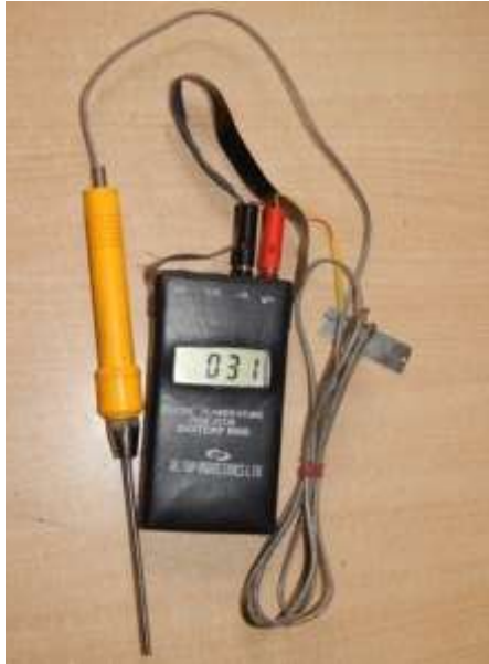
Figure 3 Thermocouple with Indicator
